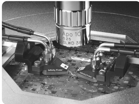
Figure 2. Dual line Infinity probe from Cascade Microtech. Available in GSGSG and GSSG configurations with pitches 100, 125, 150, 200, 225, and 250 \mu\text{m} . For more details, please contact Cascade Microtech at www.cmico.com
